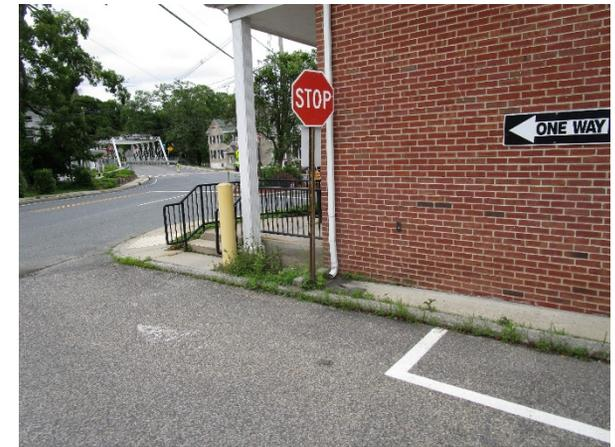
Porous pavement can be installed to collect stormwater from both the disconnected downspouts as well as from the parking lot surface. A preliminary soil assessment suggests that more soil testing would be required before determining the soil's suitability for green infrastructure.
